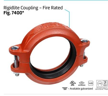
The Gruvlok Figure 7400 Rigidlite Coupling is specially designed to provide a rigid, locked-in pipe connection to meet the specific demands of rigid design steel pipe. Fast and easy swing-over installation of the rugged lightweight housing produces a secure, rigid pipe joint. The Figure 7400 Rigidlite Coupling is approved for fire protection service in both wet and dry systems, with roll grooved or cut grooved steel pipe prepared in accordance with Gruvlok grooving specifications.
